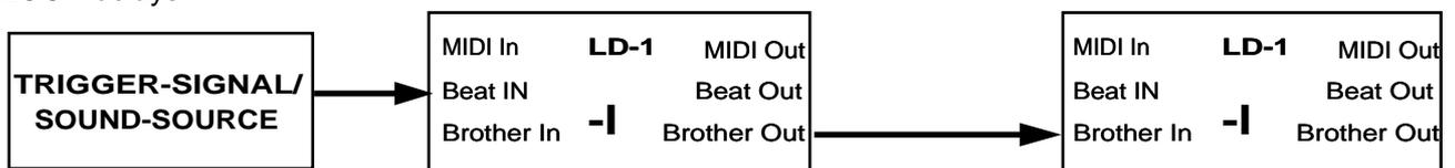
**Note!** The BROTHER SYNC does not trigger Samples (BREAK - MULTIPLY). If you want all brothers to be triggered together when they are waiting in Break, you have to connect the trigger source to all BEAT SYNC jacks or use MIDIBeatSync.
