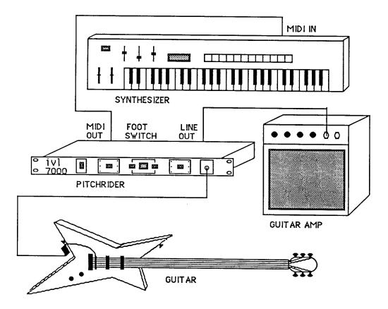
Plug the wall mount transformer into an AC outlet and plug the power plug into the rear of the unit. Now turn on the unit. The first thing to do is to check the tuning of the guitar. Play each open string one at a time. As each string is played the LED next to the corresponding string name will light.
