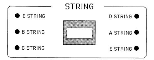
In addition to the string display, the Setting window will act as a tuning meter and show if the string is sharp or flat as follows.
