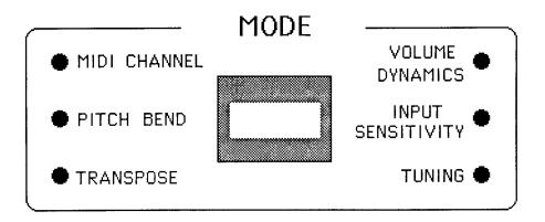
The LED indicator next to MIDI CHANNEL will light indicating that the MIDI channel that the Pitchrider transmits on can be changed. The numeric display in the SETTING window will now show the current MIDI channel selected. Immediately after power up this will be 1.
