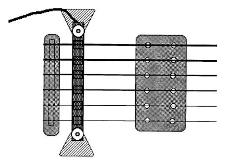
4. Cut two pieces of rubber tubing to act as springs in holding up the pickup. The length of the tubing should be just enough to push the pickup firmly up against the strings. The knurlled nuts can then be used to adjust the pickup down so that it doesn't contact the strings.
