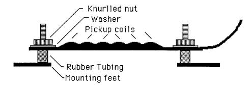
5. Slide the rubber tubing onto the mounting feet. Put the pickup under the strings, turn it on edge and slide on the mounting feet. Remove the backing from the adhesive on the feet and rotate the pickup into the normal position and stick it in place on the spot you marked in step 3. If there is limited clearance you may have to loosen the strings before you can rotate the pickup into position.
