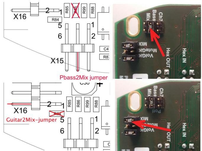
for option 5: to cut the guitar signal from the mix remove the jumper on X16pin1-2 (on boards < PB-R-0068 remove the 0-Ohm resistor R84 or move the jumper on X12 from Mix to Pbase)
